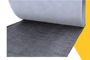
665 Membrane is 65 mil membrane composed of a self-adhering, polymer modified asphalt layer, laminated to a woven polypropylene backing. 665 Membrane is easy to work with and equally effective on bridges and pavements for waterproofing and crack control.
