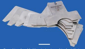
AccuTrowel is a hand held metering trowel tool set that range in size from 2"" to 12"" and are manually operated providing a means to accurately determine mil thicknesses when applying viscous coatings to pipe surfaces. AccuTrowel works perfectly with all RG-2400 products to make sure your pipe coverage is precise, and also saves material by removing any excess gel. AccuTrowel matches most standard pipe sizes and specifications.
