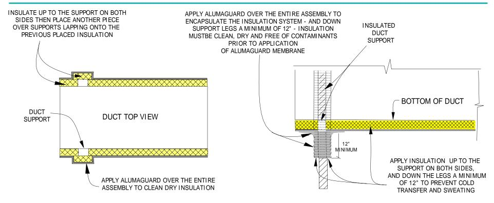
When it is not possible to lift a duct off the rooftop supports, it is necessary to incorporate the support system into the insulation system by encapsulating the supports with insulation. This same system must be used if duct supports are screwed onto the ductwork
