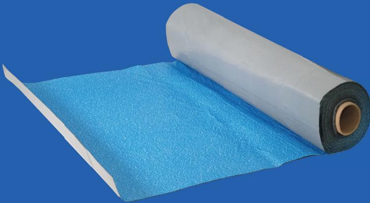
Deckguard® HT is a high heat 40-mil roofing membrane composed of a high strength slip resistant spider web backing laminated to a high performance high heat asphalt compound with a film release for ease of application. The release liner is removed leaving a strong asphalt compound to bond to the roof deck.
