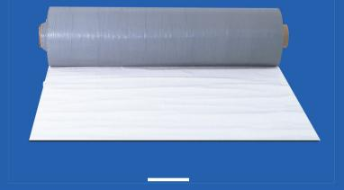
Insulrap JB is a self-adhesive multi-layer white PET/FOIL/-PET zero perm membrane designed specifically for LNG and Cryogenic insulation systems. The product is constructed of a proprietary Polyguard butyl compound, which is a peel and stick self-sealing with excellent low temperature adhesion and flexibility, it can be installed down to 0°F.
