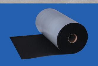
NW75 Membrane is comprised of a non-woven polypropylene fabric laminated to a rubberized asphalt waterproofing sealant-adhesive. NW75 seals and waterproofs joints and cracks, as well as bridge decks when installed following Polyguard installation guidelines. The open fibers of the non-woven geotextile fabric provide a mechanical bond to the new asphalt overlay, while the rubberized asphalt sealant-adhesive bonds to the existing pavement surface.
