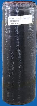
*Polyflow<sup>®</sup> 18 Drainage Mat is two-part, molded sheet drainage geocomposite consisting of a formed impermeable polymeric core covered on one side with woven filter fabric. The fabric allows water to pass into the drain core while restricting the movement of soil particles which might clog the core. The core allows the water to flow to designated drainage exits. Polyflow 18 is designed for horizontal applications. Compressive strength is 21,000 psf.*
