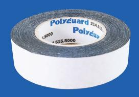
VaporGuard™ Butyl Tape is a non-curing elastomer developed for use as a vapor stop on sub-freezing insulation systems. This product provides excellent cold temperature flexibility at -20°F. System design includes installation under the insulation at terminations and in-line vapor stop locations, or expansion joints. VaporGuard retards moisture ingress along the pipe and into the insulation system at terminations and insulation
