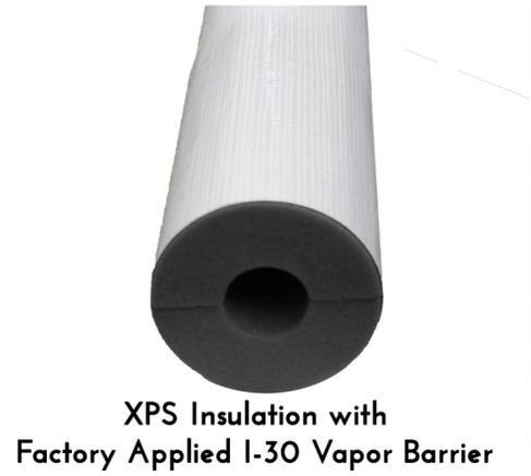
**Single layer insulation systems (Cold Service)** On the medium temperature side of the cold system temperature range, single layers are common. On Chilled Water application and sometimes on the high temperature side of cold service (0°F to 25°F) it is common to install a single layer of insulation but with offset butt joints and joint sealant on all joints. The moisture drive is becoming very intense so more precautions are necessary.
