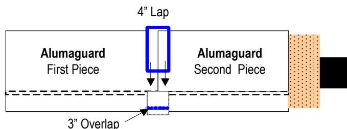
**NOTE:** Care should be taken when using **Alumaguard®** products on hot systems to insure that the surface temperatures after insulation do not exceed our upper use limitations. It is important to note that heat transfer through single layer joint seams could result in the softening or melting of the rubberized asphalt compound.
